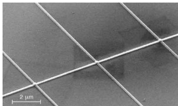
**Figure 4.** A SEM image of a 1D circuit of MSTJs (scale bar 2  $\mu\text{m}$ ). Each junction has an area of 0.007  $\mu\text{m}^2$  and contains about 5000 molecules. The inter-wire separation distance was kept large so as to simplify the task of contacting this circuit to external devices for testing.
