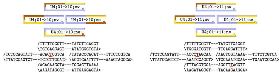
Figure S9.1: Naming conventions for tile strands. Two example proofreading blocks are shown, each with their corresponding four DNA strand sequences laid out graphically below. Brown represents bit 0 and yellow represents bit 1. Red-underlined T bases have a /iBiodT/ (biotin) modification. Blocks and tiles are named as follows. First, note that Figure S10 of Supplementary Information A shows proofreading blocks being positioned along rows named U1 to U8, and how those row names correspond to wire numbers of a 6-bit IBC (Figure 1a in the main text shows two wires there named w1 and w2). Using this convention each proofreading block is named by (a) the unique row it appears in, e.g. U4), and (b) the function it computes (e.g. 01->10), so an example proofreading block name is U4;01->10. Tiles within a block are then identified by their proofreading block and a pair of letters: sw , se , ne , or nw . The “_” symbol indicates a tile domain that does not encode a bit as it is in, or binds to, the seam block.
