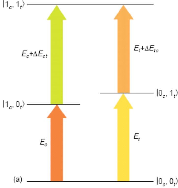
Figure 4: The CNOT gate which flips the target bit only when the control bit is 1 [15].
