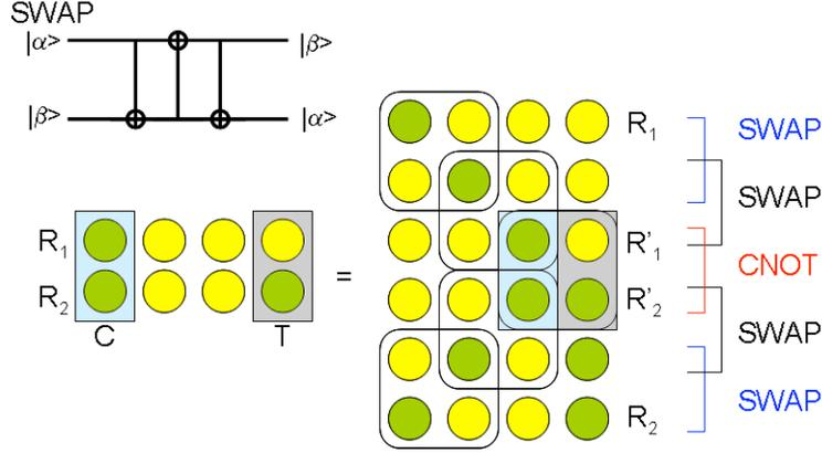
Figure 5: The SWAP gate which swaps the two input qubits. SWAP can be realized by taking three CNOT gates operations. This gate is essential when we want to perform operations on remote qubits such as the CNOT gate shown above [15].
