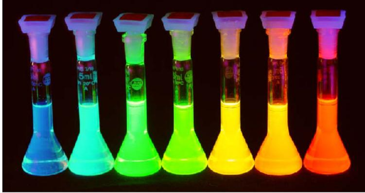
Figure 1: Colloidally prepared CdSe quantum dots of different sizes, demonstrates how the size of the quantum dot affects confinement and thus the optical properties of the material [11].
