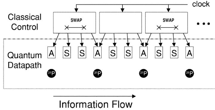
Figure 10: Swapping channel quantum data path [29].
