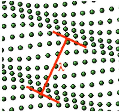
Figure 13: A longitudinal vibration (sound wave) propagating through a crystal lattice (reproduced from Wikipedia.org)
