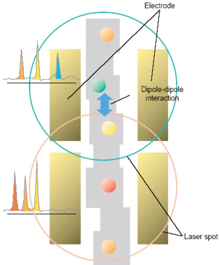
Figure 2: Linear array of quantum dots for all-optical computation. Individual QDs are accessed and distinguished by positioning the tunable laser and probe. The statistical distribution of QD characteristics enables the identity of an exciton in a particular QD to be recognized by frequency domain discrimination [15].
