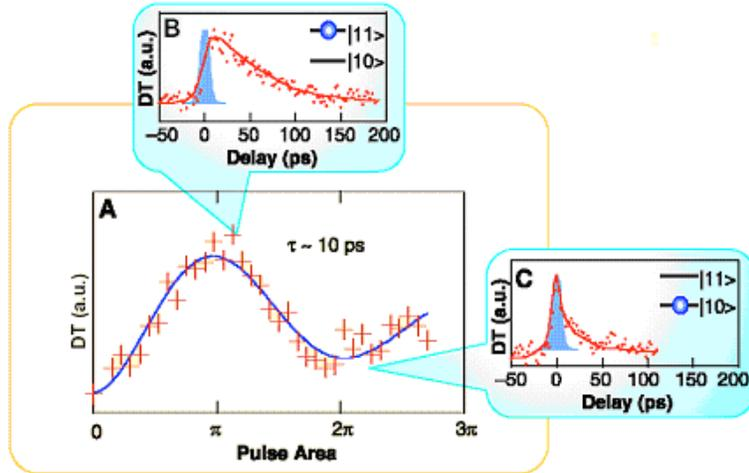
Figure 8: Biexcitonic Rabi oscillations. (a) Measured differential transmission (DT) vs the pulse area at fixed time delay  $\tau$  10ps, a sine-squared function with exponentially decaying amplitude (b and c) DT vs. time delay at fixed pump powers. The target states that follow the pump pulse are shown in the upper right, where the circles represent the exciton population [20].
