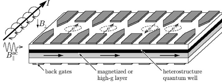
Figure 11: Theoretical proposal for defining quantum dots by using electrical gating. [33]. The magnetic fields shown in the diagram are representative of an ESR technique [35] for single-spin rotation.
