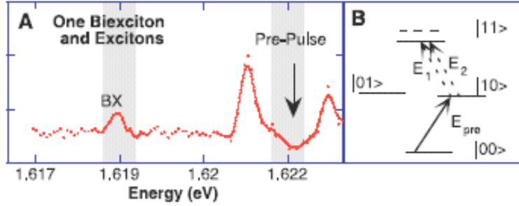
Figure 7: (a and b) The spectrum and experimental configuration with a pre-pulse tuned to one exciton transition and the biexciton (BX) state appearing at the lower energy end [20].
