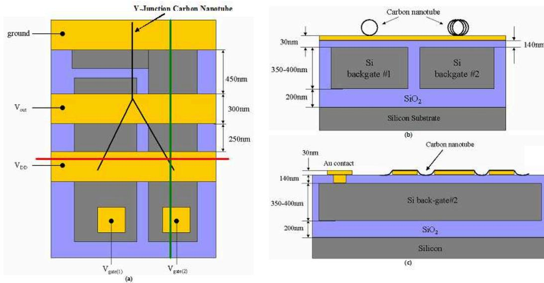
Figure 22: The final Y-branch NAND device. (a) Top-down view (b) Cross-section along the red line (c) Cross-section along the green line.
