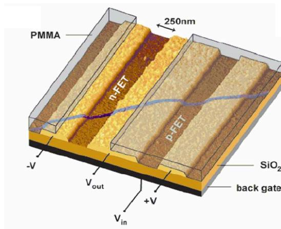
Figure 10: Intramolecular Inverter
