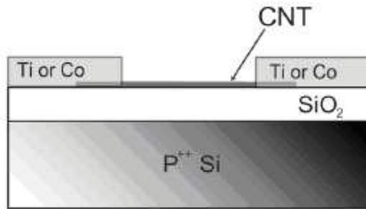
Figure 9: Schematic cross-section of the improved CNT-FET
