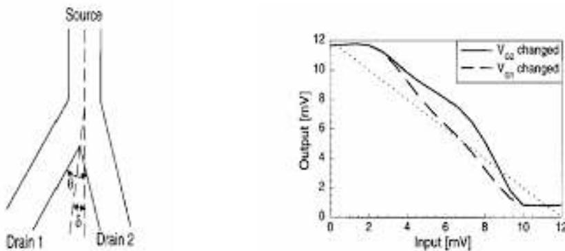
Figure 20: (left) asymmetric Y branch needed for NAND device (right) voltage characteristics of NAND gate [10]
