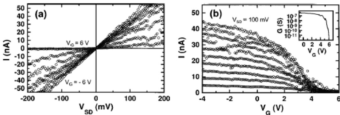
Figure 8: output and transfer characteristics for a CNT FET with 30 nm thick Au electrodes and a single-walled nanotube of 1.6 nm diameter [1]. (a) shows  $I - V_{SD}$  curves measured for  $V_G = -6, 0, 1, 2, 3, 4, 5, 6V$ . (b) shows  $I - V_G$  curves for  $V_{SD} = 10 - 100mV$  in steps of  $10mV$ . The inset shows that the gate modulates conductance by 5 orders of magnitude.
