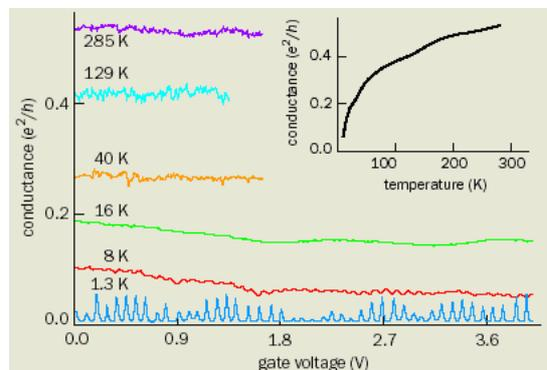
Figure 4: conductance of metallic nanotubes at six different temperatures as a function of gate voltage; average conductance slowly decreases as temperature is lowered. [6]
