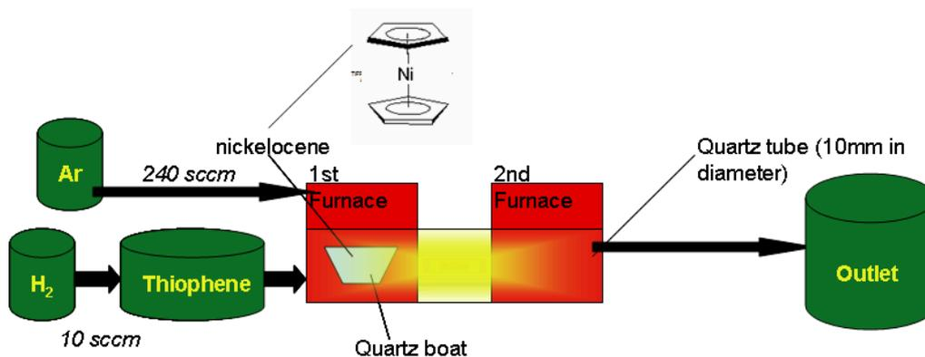
Figure 12: the scheme of pyrolysis method of fabrication Y-junction carbon-nanotubes
