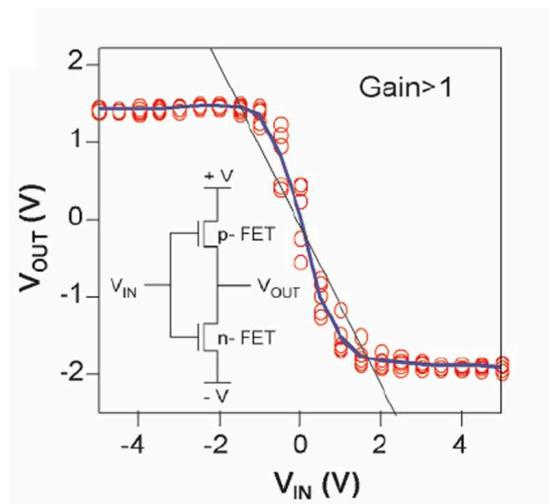
Figure 11: Intramolecular inverter measurements
