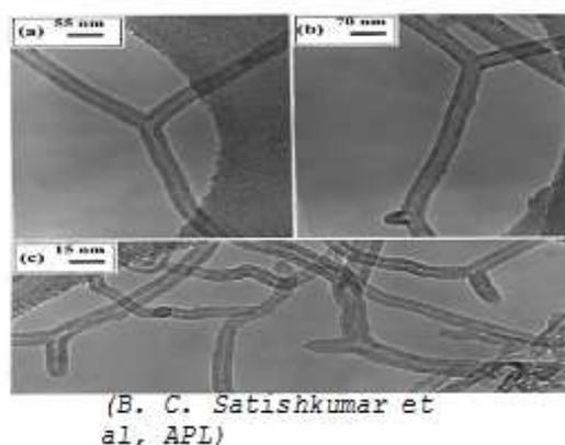
Figure 13: TEM image of a Y-junction carbon nanotube
