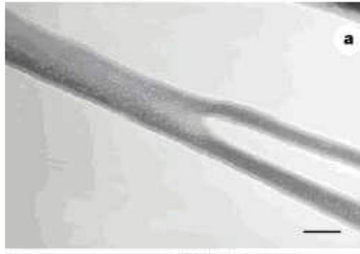
Figure 14: Y-junction tube (scale bar,  $50\text{nm}$ ) with stem  $90\text{nm}$  and branches  $50\text{nm}$  in diameter.
