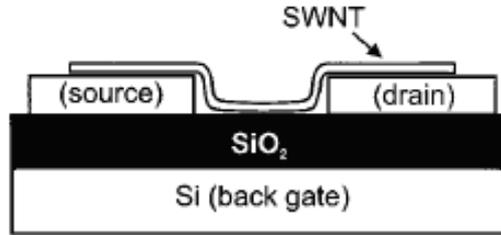
Figure 7: Schematic cross section of a SWCNT FET
