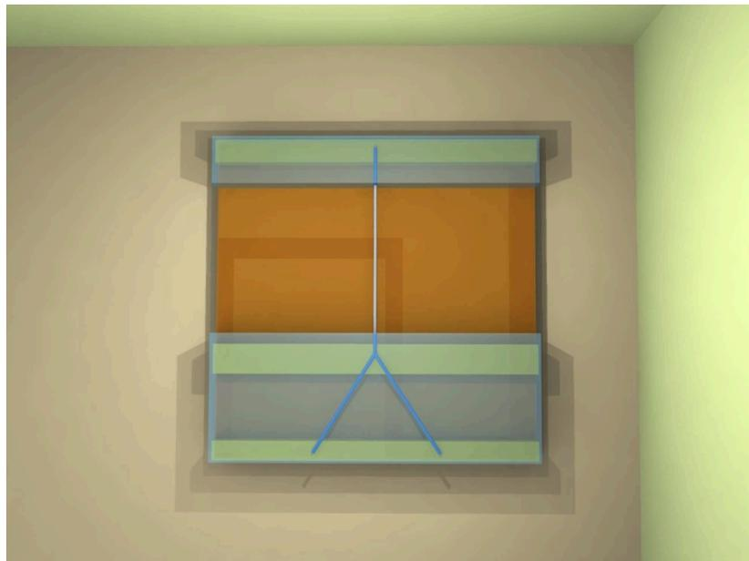
Figure 23: Top-down view of the PMMA-protected and potassium-doped nanotube NAND gate device
