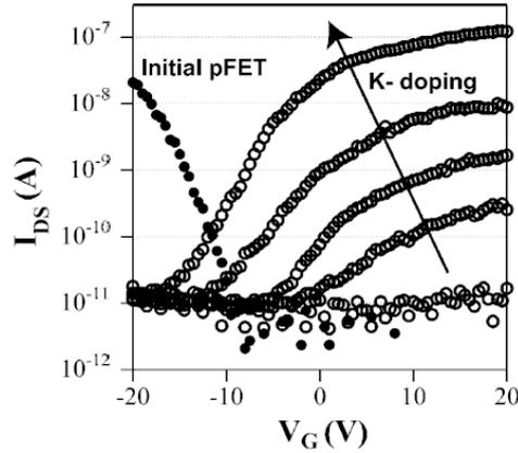
Figure 6: changing output characteristics of CNT field effect transistor being doped with potassium [5]
