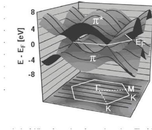
Figure 2: Electronic Band Structure of 2D graphene sheet; six K-points lying at Fermi energy are shown as well as the first Brillouin zone [5]
