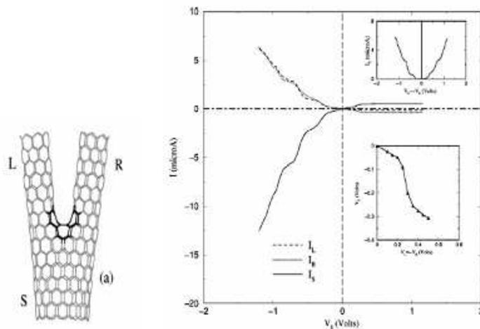
Figure 17: (left) symmetric Y branch (right) graph of current through stem,  $I_S$ , and branches  $I_L$  and  $I_R$ ; current is positive flowing towards junction and negative otherwise. This figure shows rectifying behavior. [9]
