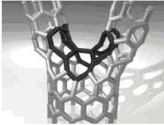
Figure 15: Y branch nanotube; topological defect of carbon nanotube [8]
