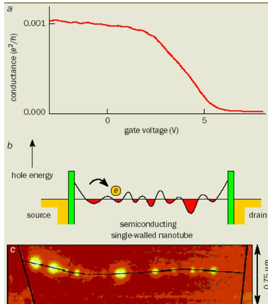
Figure 5: (a) conductance of semiconducting nanotube as function of gate voltage (b) potential profile of disorders experienced by holes due to impurities in structure of the nanotube (c) STM measuring nanotube conductance [6]
