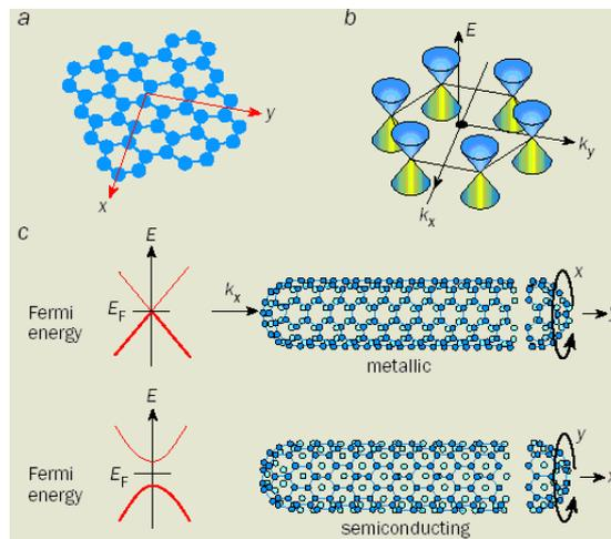
Figure 3: (a) lattice graphene (b) energy conducting states in graphene as function of wavevector  $k$  (band structure of nanotube would then be 1D slices through the 2D bandstructure) (c) graphene rolled around  $y$  axis results in metallic nature, rolled around  $x$  axis results in semiconducting nature. [6]
