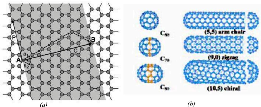
Figure 1: (a) generating chirality vector for nanotube from graphene sheet.  $C = na_1 + ma_2 = (n, m)$ , where  $a_1$  and  $a_2$  are unit vectors of the hexagonal lattice. [5] (b) Various carbon nanotubes resulting from different foldings of graphene sheets
