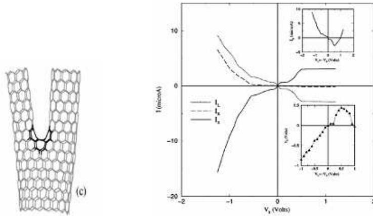
Figure 18: (left) asymmetric Y branch (right) graph of current through branch showing typical interconnect behavior, no rectification. [9]
