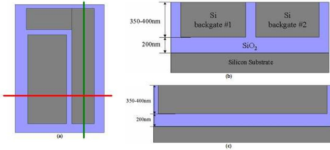
Figure 21: The patterned silicon back-gates. (a) Top-down view (b) Cross-section along the red line (c) Cross-section along the green line.
